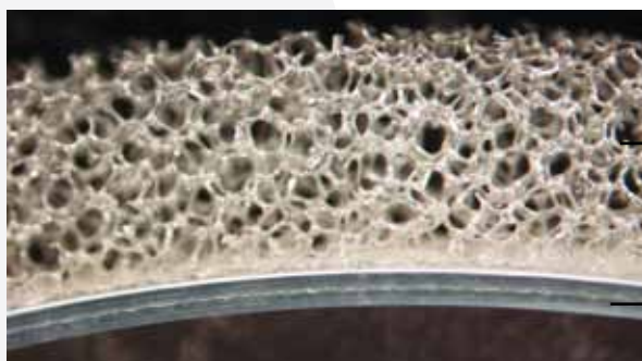
Lateral view of an implant shell with Microthane ® coating
